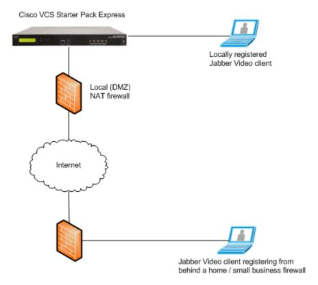
If the VCS Starter Pack Express services endpoints that are behind a firewall, the VCS could be configured with a public IP address and the local (DMZ) firewall would have to be configured to pass the specific public IP address traffic to the VCS.
