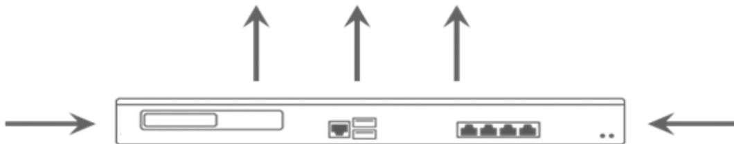
Figure 1: Cisco VCS ventilation
